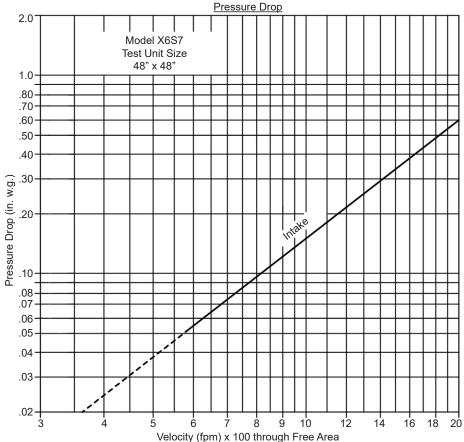
Intake air converted to standard air density.
